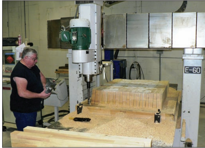
Master builder Louis Wharton, a 37-year Fabri-Form employee, refinishes a mold block at the New Concord, Ohio, tool shop.
